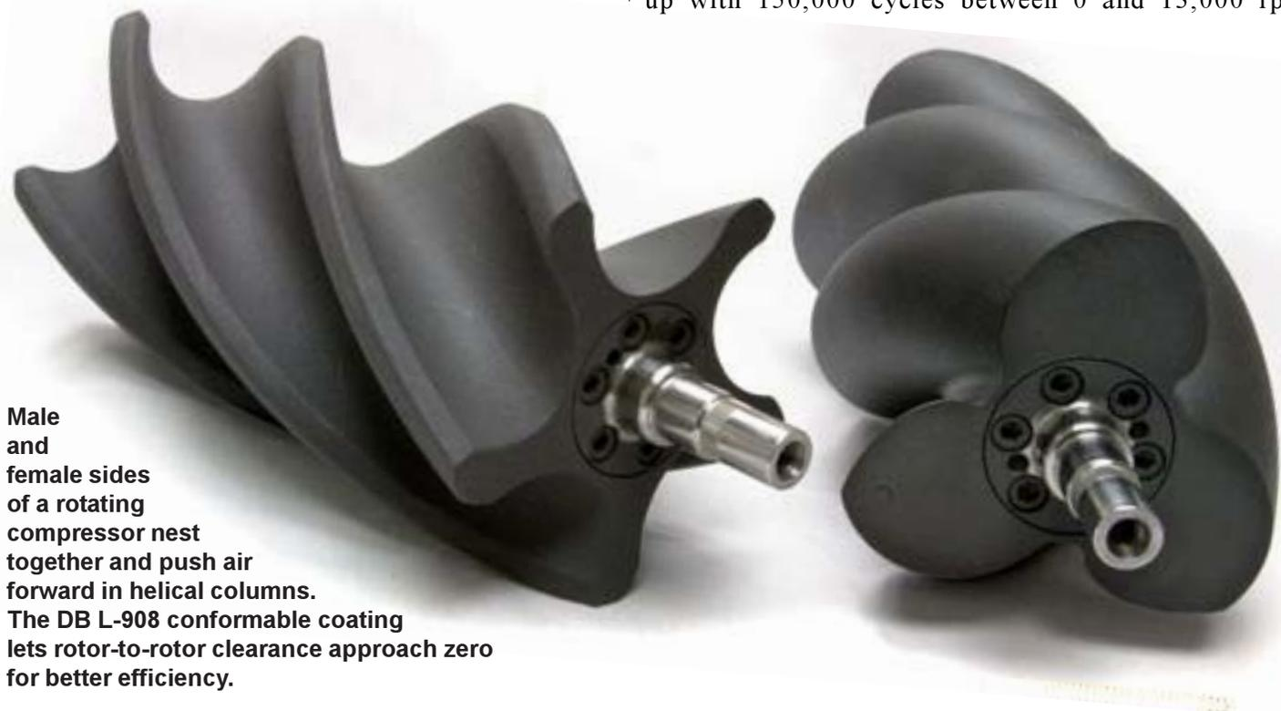
**Male and female sides of a rotating compressor nest together and push air forward in helical columns. The DB L-908 conformable coating lets rotor-to-rotor clearance approach zero for better efficiency.**
